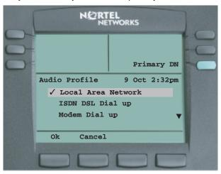
You can toggle between enabling the Audio Local Area Network functionality by pressing the down navigation key. Press **Ok** to save the setting and return to the Main menu. Press **Cancel** to return to the Audio Profile screen without saving your changes.
